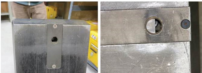
Example of a shutter fully open (left) and a shutter that is half-open (right)
